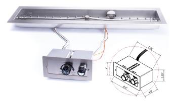
Push button fire pits are controlled using a simple knob and button on a stainless steel valve box and features a flame-sensing system to turn off gas if flame is lost.
