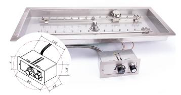
Push button fire pits are controlled using a simple knob and button on a stainless steel valve box and features a flame-sensing system to turn off gas if flame is lost.
